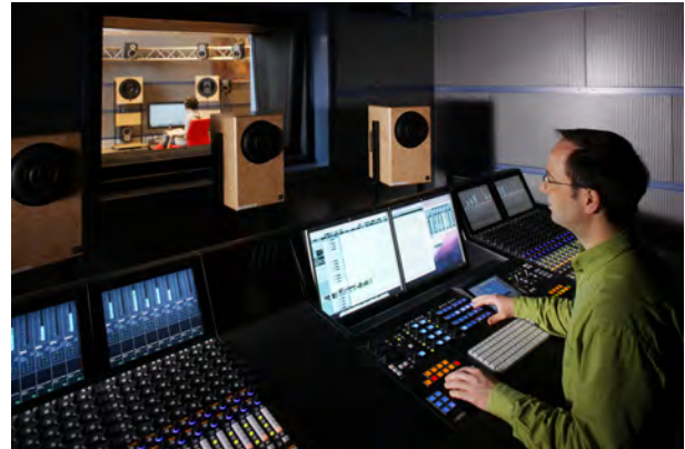
Figure 17: Universal mixing controller without audio processing in Strawinsky. View through the window into Mozart.
